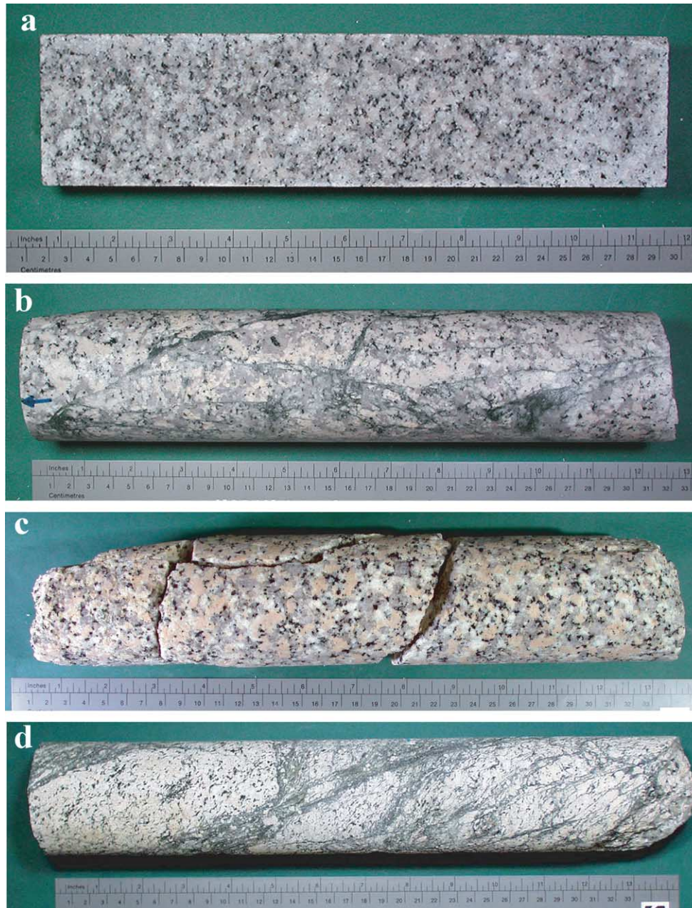
Fig. 4. Examples of the drill core samples. (a) Fresh and undeformed granite in domain A. Sample 113, depth 350 m from the ground surface. (b) Fractured granite in domain B intruded by cataclastic seams. Sample 188, depth 575 m. (c) Fractured granite in the fault damage zone of domain C. Sample 229, depth 698 m. (d) Foliated cataclasite in domain D at the center of the Tsukiyoshi Fault. Sample 332, depth 707 m.
